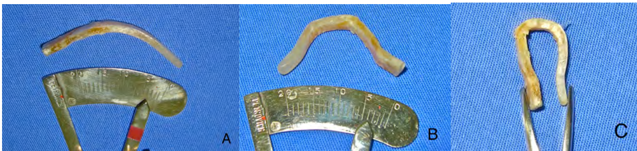
Fig 2: Spring, left open(A) , middle molded (B), right in compression (C).
