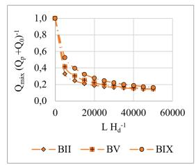
**Figure 5.** Peak flow attenuation through the downstream channel - 10 m dams.
