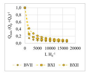
**Figure 7.** Peak flow attenuation through the downstream channel - 30 m dams.
