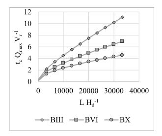
**Figure 12.** Dimensionless relation of the arrival time of the peak discharge - 15 m dams.
