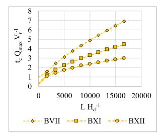
**Figure 13.** Dimensionless relation of the arrival time of the peak discharge - 30 m dams.
