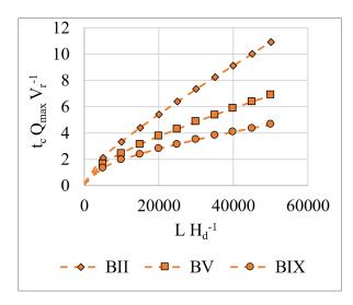
**Figure 11.** Dimensionless relation of the arrival time of the peak discharge - 10 m dams.
