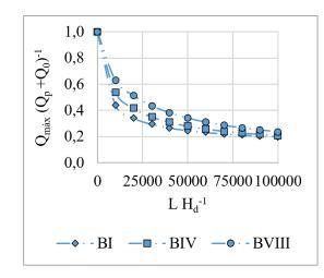
**Figure 4.** Peak flow attenuation through the downstream channel - 5 m dams.
