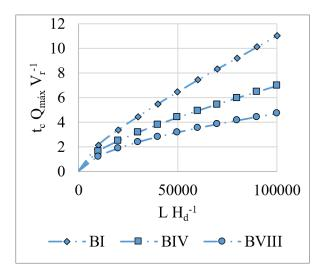
**Figure 10.** Dimensionless relation of the arrival time of the peak discharge - 5 m dams.
