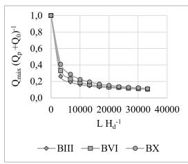
**Figure 6.** Peak flow attenuation through the downstream channel - 15 m dams.
