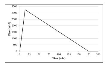
Figure 16. Case study breach outflow hydrograph.
