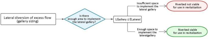
Figure 4. Prerequisites relating to the river margins in the river revitalization process.
