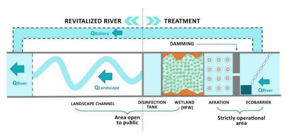
Figure 2. Configuration of flows in the project layout.
