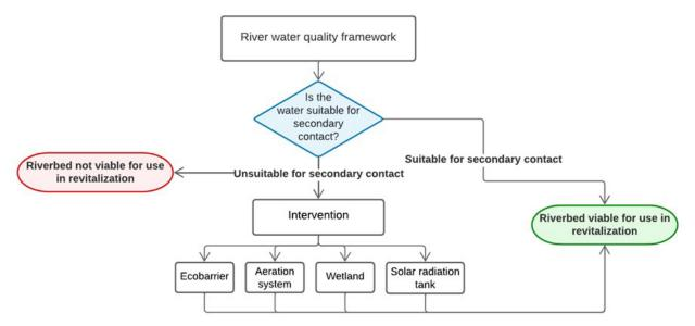
Figure 3. Pre-requisites regarding the water quality assessed in the river channel of the river revitalization process.
