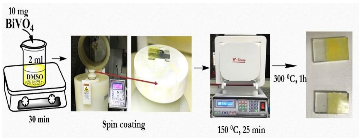
Figure 2. 4. Synthesis process of W:BVO, W:BVO/FeNiO x , and W:BVO/FeMnO x films.
