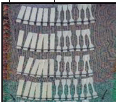
Figure 2 – PP specimens, with and without benzoin, exposed to natural weathering in Porto Alegre/RS.
