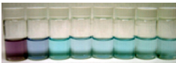
Figure 13. Biuret test of the protein solutions (1 to 8, from left to right).
