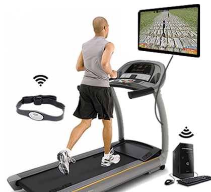
Figure 1: System overview. Running Wheel captures heart beat rhythm wirelessly and treadmill speed. This information is recorded and used in a motivational exergame to improve performance.
