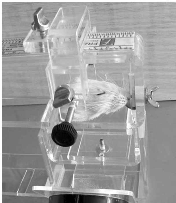
Figure 1. Rat head positioned in apparatus.
