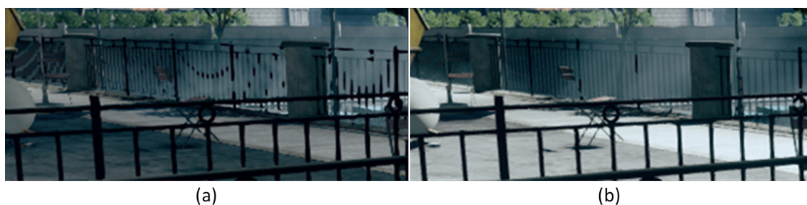
Figure 4.8: Aliasing example: complex details. (a) in the back fence, we see patterns artifacts, characterizing Moiré effect, due to improper sampling. (b) with improved sampling AA, the back fence is better represented (image from (BATTLEFIELD, 2014)).
