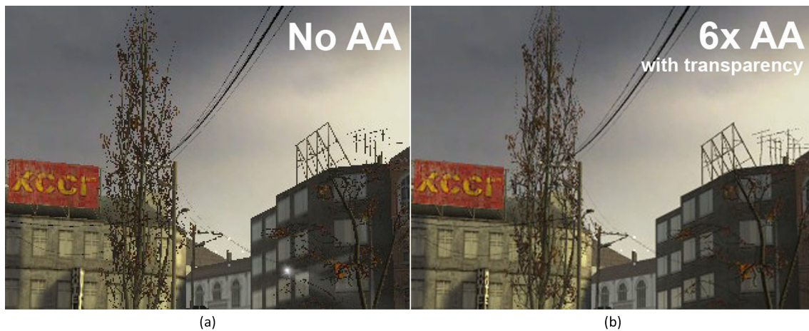
Figure 4.7: Aliasing example: discontinuity. (a) without AA, we see elements of the scene generating discontinuities: power cables and pole, trees, antennas and outdoor supports. (b) these problems are alleviated through AA, providing a more meaningful image (image from (GTA, 2012)).
