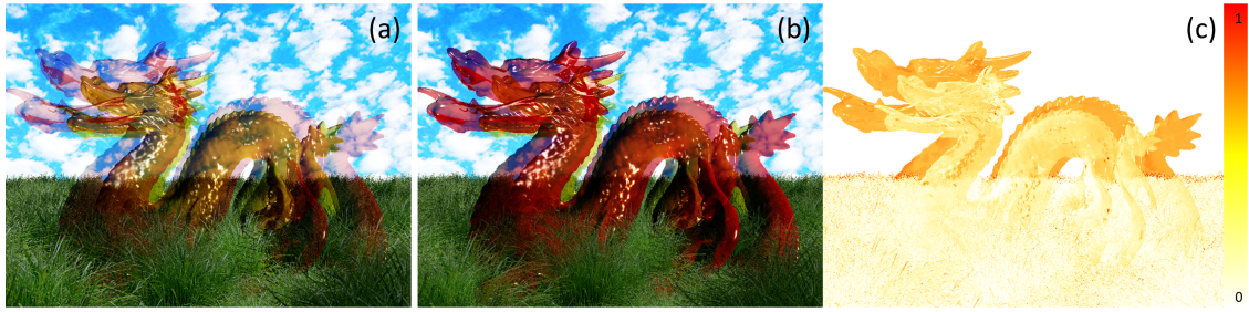
Figure 3.30: Transparent scene with different opacities: the opacity for the red dragon is 0.15, and for the yellow dragon is 0.3; the grass uses alpha texture with opacities varying from 0 to 1. (a) correct blending with individual alpha per fragment ( R_8G_8B_8A_8Z_{32} ); (b) image rendered with a global alpha for all fragments (mean alpha of the scene = 0.3 ( R_{32}G_{32}B_{32}Z_{32} )); (c) error when rendering with global alpha (RGB distance mapped in color codes).
