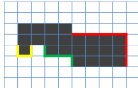
Figure 4.13: Examples of L (red), Z (green) and U (yellow) shapes detected in an aliased image by the MLAA technique.
