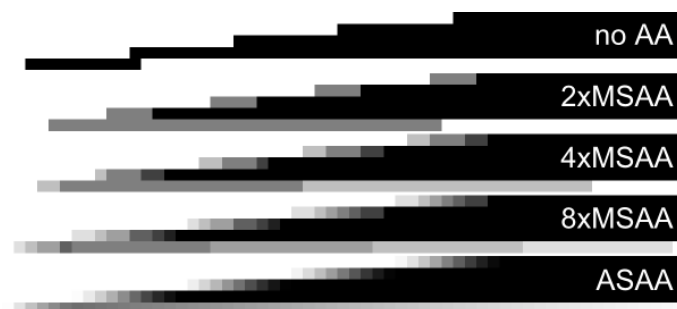
Figure 4.15: Our accelerated area-sampling approach produces superior edge-AA. Point-sampling approaches rasterize S samples per-fragment, so they can generate up to S shades of color transition. This results in blocks of pixels with the same shade and abrupt color transitions between these blocks. Our proposed area-sampling generates smoother color transition while rasterizing only one sample per fragment. Because of its ability to capture smaller variations on pixel coverage, ASAA can paint each pixel with a different shade; compare the gray lines on the bottom of each method.
