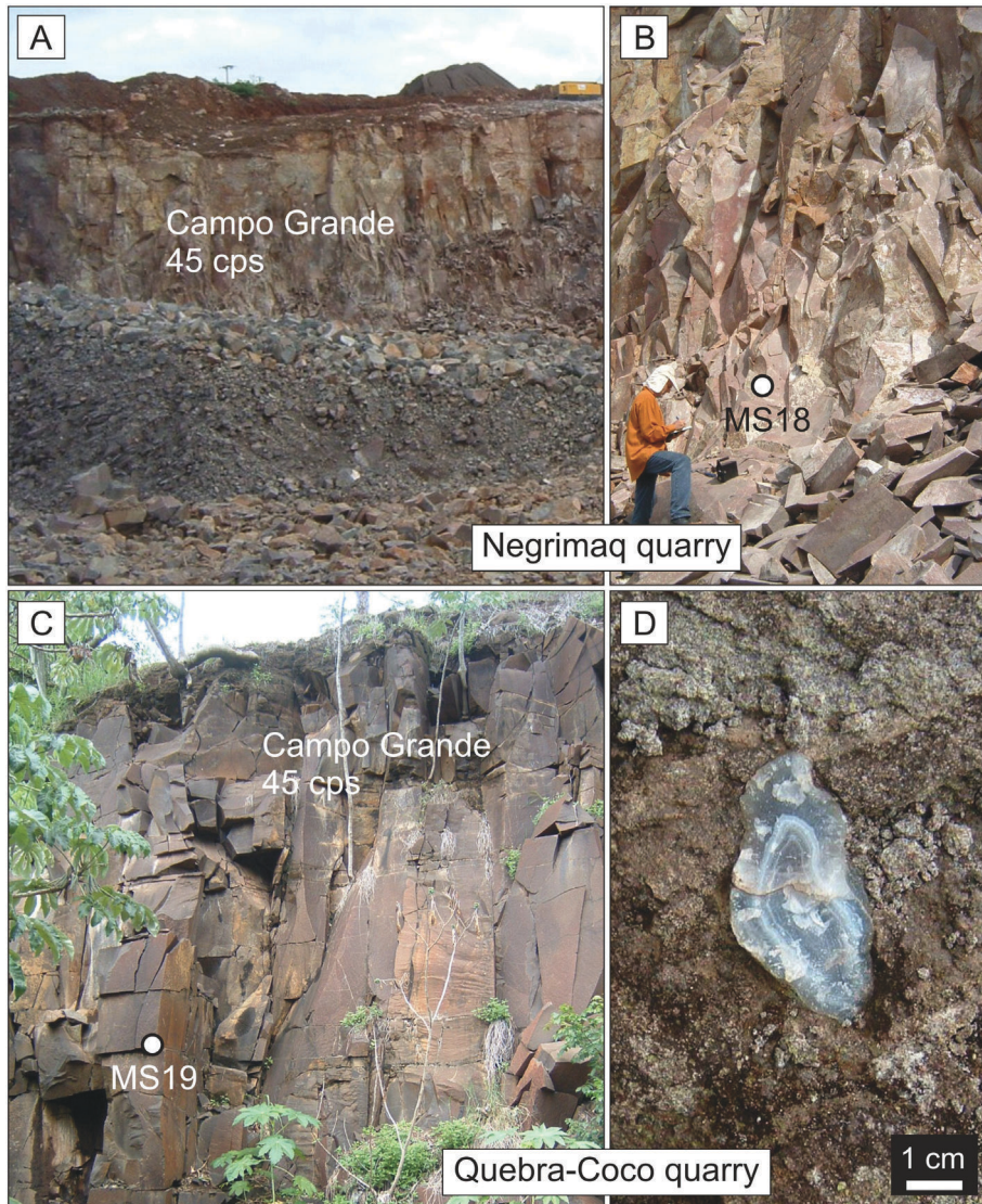
Fig. 6. Field photos of Negrimaq and Quebra-Coco quarries. Flow names (e.g., Campo Grande) and sampling sites of chemical analysis rocks are indicated (e.g., MS19). A) Negrimaq quarry; B) columnar jointing in Negrimaq quarry; C) Quebra-Coco quarry; D) Agate geode in the Quebra-Coco quarry.
