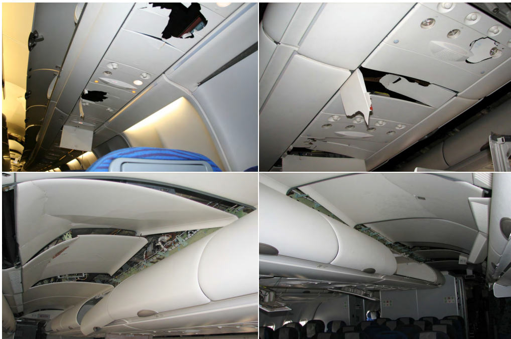
Figure 1.2: Resulting damage to airplane from impact with persons and objects.
