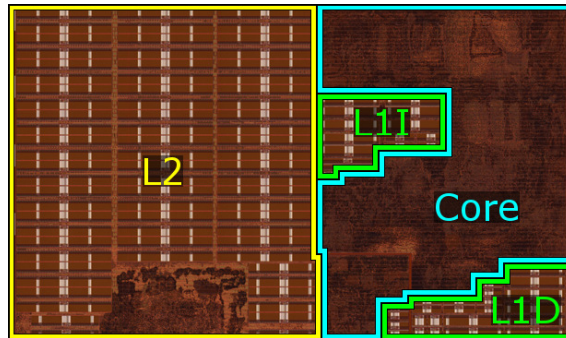
Figure 5.1: Approximate area of essential resources for computation (Core) and extra resources used to speed-up execution (L1 and L2 Caches) marked on a polysilicon die photo of a Cortex-A9 with 32 KB Instruction/Data L1 Caches and 512 KB L2 Cache.
