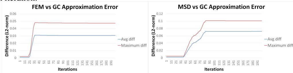
Figure 6.13: Effectiveness evaluation of first scenario. On the left, comparing the error by using GC to approximate FEM, and on the right the error by using GC to approximate MSD. The dimensions of the cylinders (after applying the gravity) are: width=1.24 , height=1.72 , and depth=1.24 . We have recorded the average and maximum errors for each iteration.
