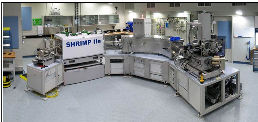
Figura 13 - SHRIMP da Australian National University em Canberra – Austrália (extraído do site: http://www.ga.gov.au/energy/disciplines-techniques/geochronology.html acessado em: 01/09/2011 )
