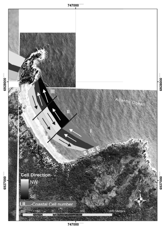
Figure 13: Coastal cells direction (gray tonalities indicate variation in current speed,- the extremes of color palette represents the higher velocities for each direction) in the Matadeiro Beach. The shoreline is differentiated in grey colors to represent the coastal cell boundaries.
