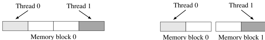
(a) Low granularity. The data accessed by the threads belong to the same memory block.
