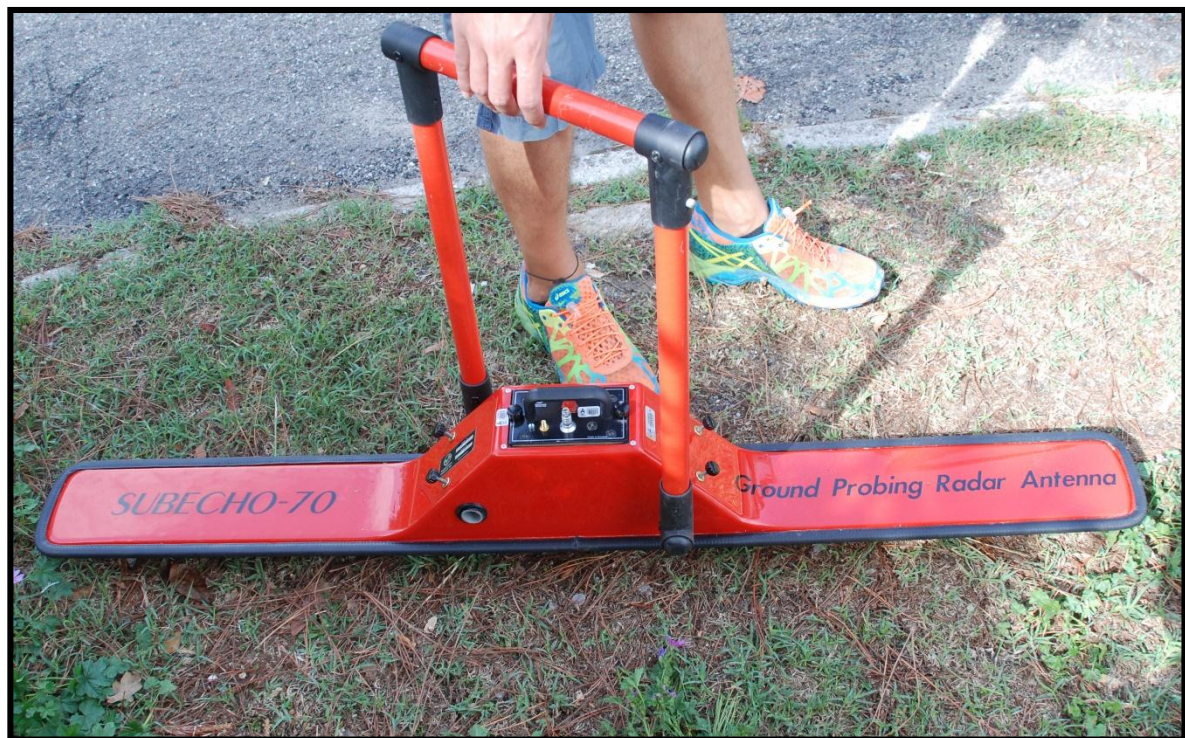
Figure 11: The GPR antenna used to acquire the subsurface data in the Ravenna Coastal Plain.
