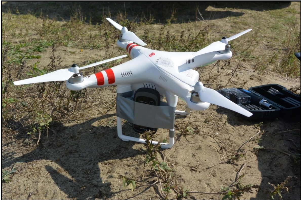
Figure 12: The DJI Phantom 2 with the eTrex ® 30-Garmin GNSS attached to the UAV to increase the georeferencing accuracy.
