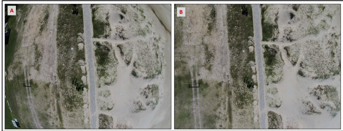
Figure 13: Aerial photos from DJI Phantom 2. A) The aerial photo before correction; B) the aerial photo after the profile correction.
