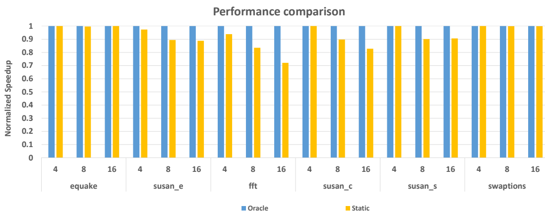
Figure 7.19: Performance comparison between the Oracle and the Static schedulers. The speedup is normalized to the Oracle’s performance. The static scheduler can reach near Oracle performance on very unbalanced applications (due to most of the work being executed on a large core) and very balanced applications (as all cores execute the same load, no scheduling is necessary).
