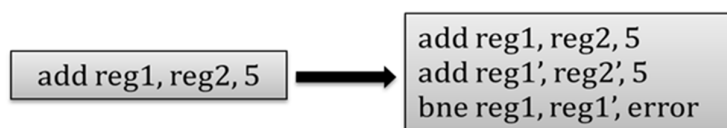
Fig. 2.5: Example of a SIHFT technique.
