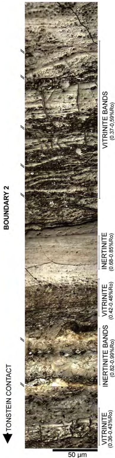
Fig. 6. Composite image of petrographic observation and reflectance values of boundary 2 (Pb467T). \\\ = content of mineral matter has been omitted from the image composition due to space constraints.
