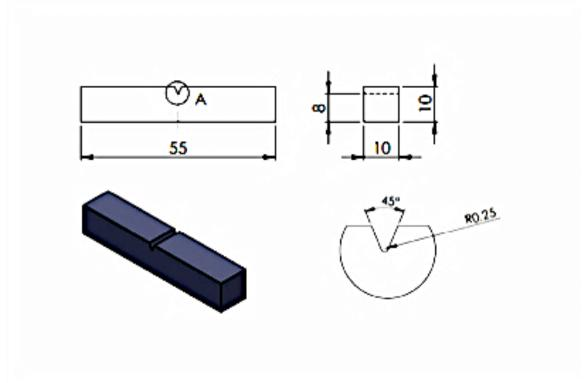
Figure 1. Test specimens, dimensions in millimeters.
