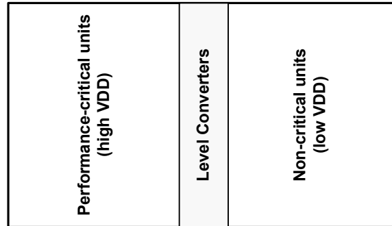
Figure 2.6: Two-level multiple static supply voltage scheme.
