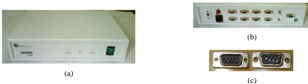
Figura 28. (a) Console de controle SEEPAV 8200, (b), painel traseiro SEEPAV 8200 e (c) conector serial. Fonte: Malysz (2009)
