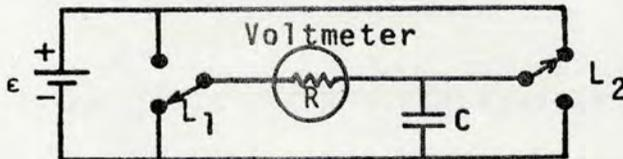
In this position, the capacitor charges itself almost instantaneously because its terminals are directly connected to the source.
