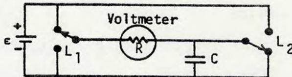
In this circuit, when the switches  $L_1$  and  $L_2$  are closed as in the figure, the voltmeter indicates the source tension  $\epsilon$ .
