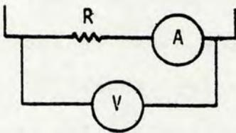
In this case, the ampermeter will only indicate the current through the resistor but the voltmeter will indicate the electric tension applied on both the resistor and the ampermeter. You must choose the best one from the two possible circuit connections; in any case, however, never connect the ampermeter in parallel with the electric source.
