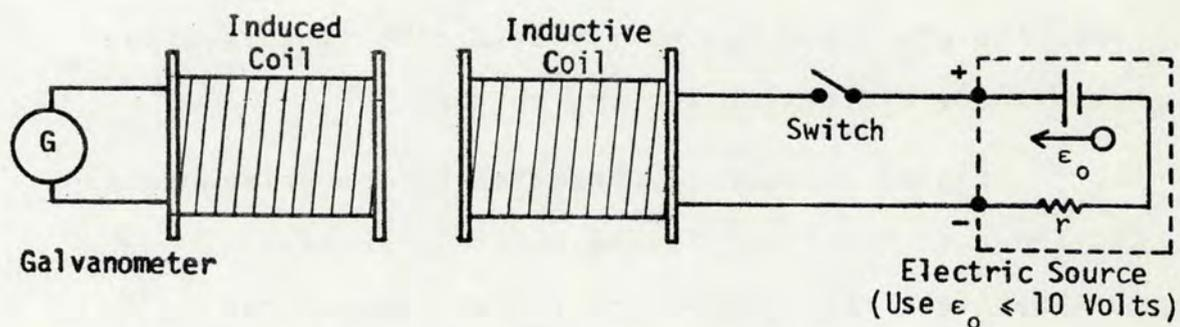
With this experimental device you can study the induced electric current in function of the relative motion between the coils, the velocity of this motion, the relative positions between the coils by putting them in several positions when closing and opening the switch; in function of the intensity of the inductive magnetic field, the distance between the coils, the relative angular position of the
