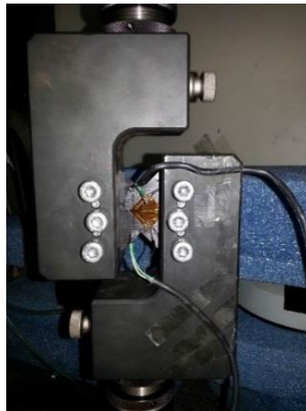
Figure 23. V-notched shear test with a bonded rosette.
