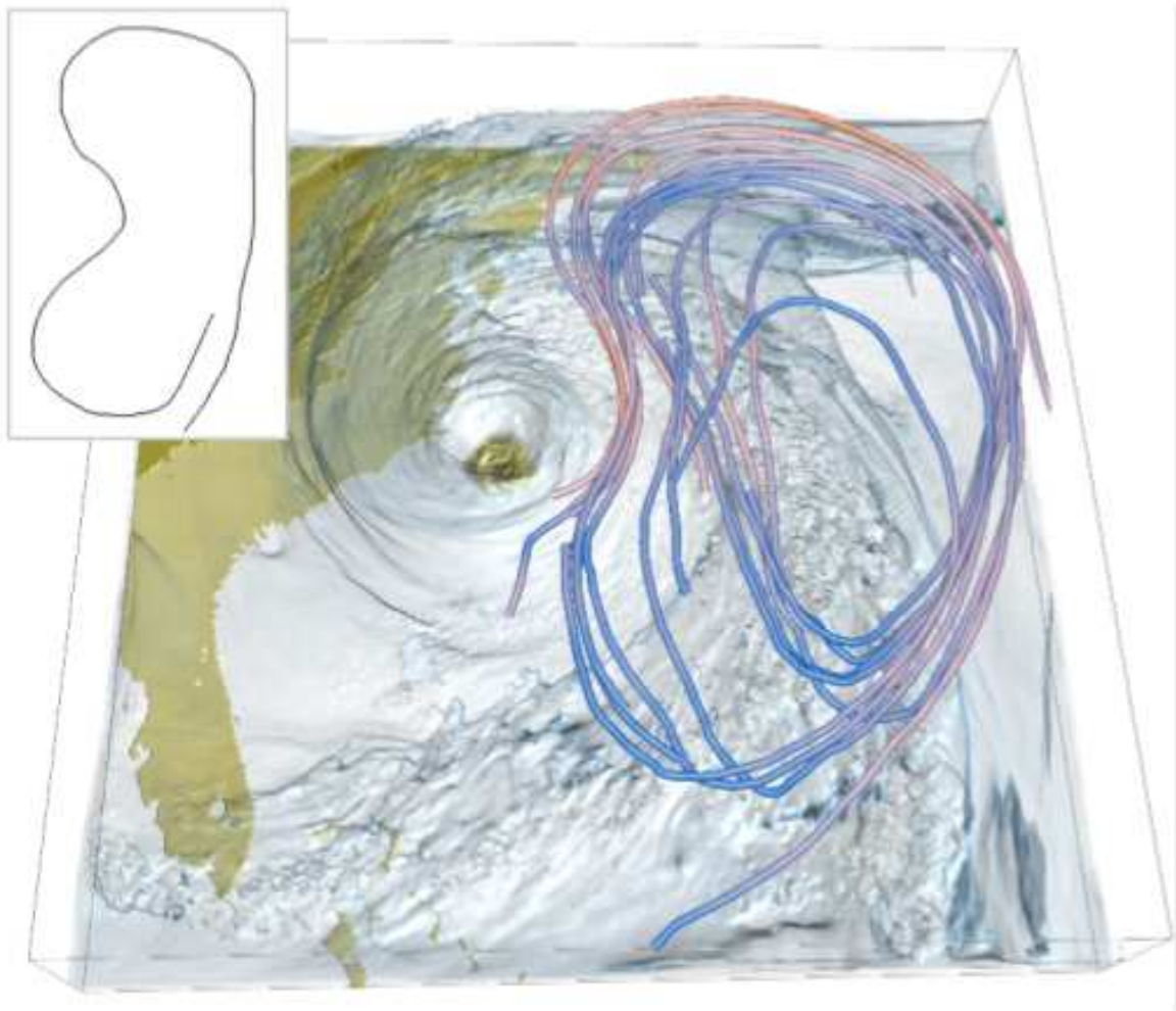
Figure 3.4 – A sketch-based clustering using template query. The user sketches an ellipse pattern (top left), and the matching streamlines are identified and displayed.
