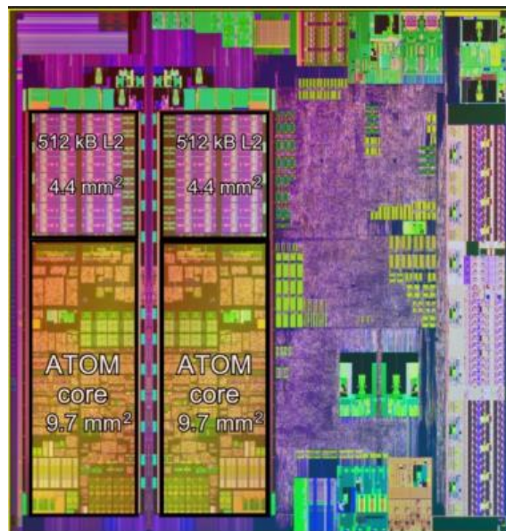
Figure 4.3: Layout of Intel Atom 45nm dual-core processor (CHIP-ARCHITECT, 2010).
