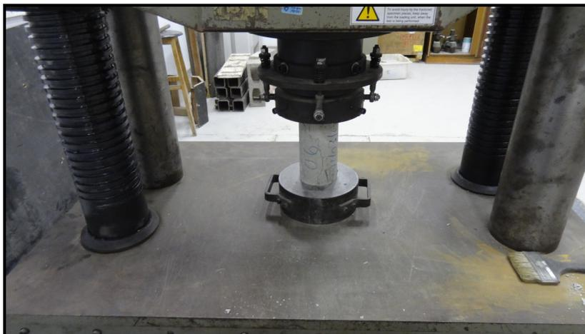
Figura 4.21 – Ruptura do CP6
