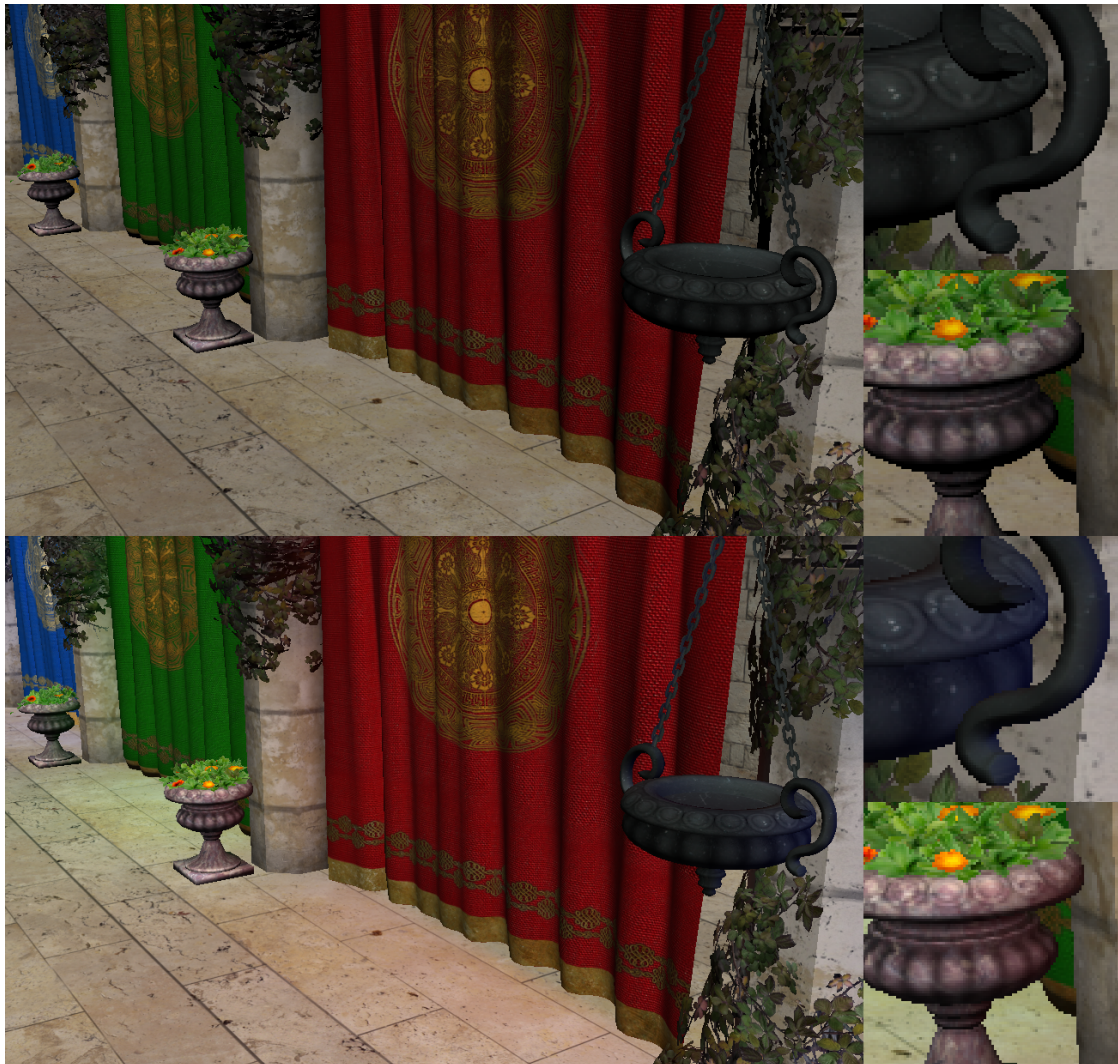
Figure 5.3: Comparison between direct illumination only (top) and direct plus indirect illumination (bottom) on the Sponza test scene showing close-up details of the color bleed in the scene (different position)
