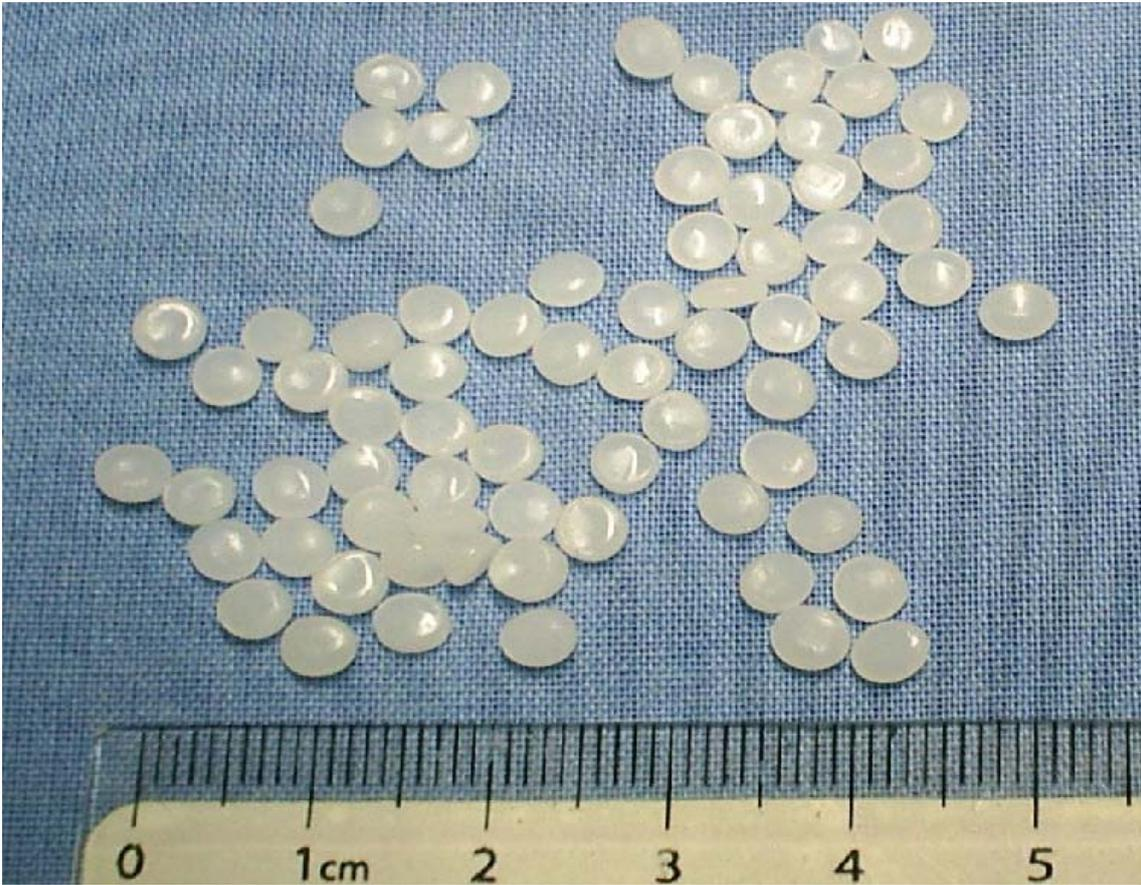
Figure 2: High density granulated polietilene used in the infusion placebo.
