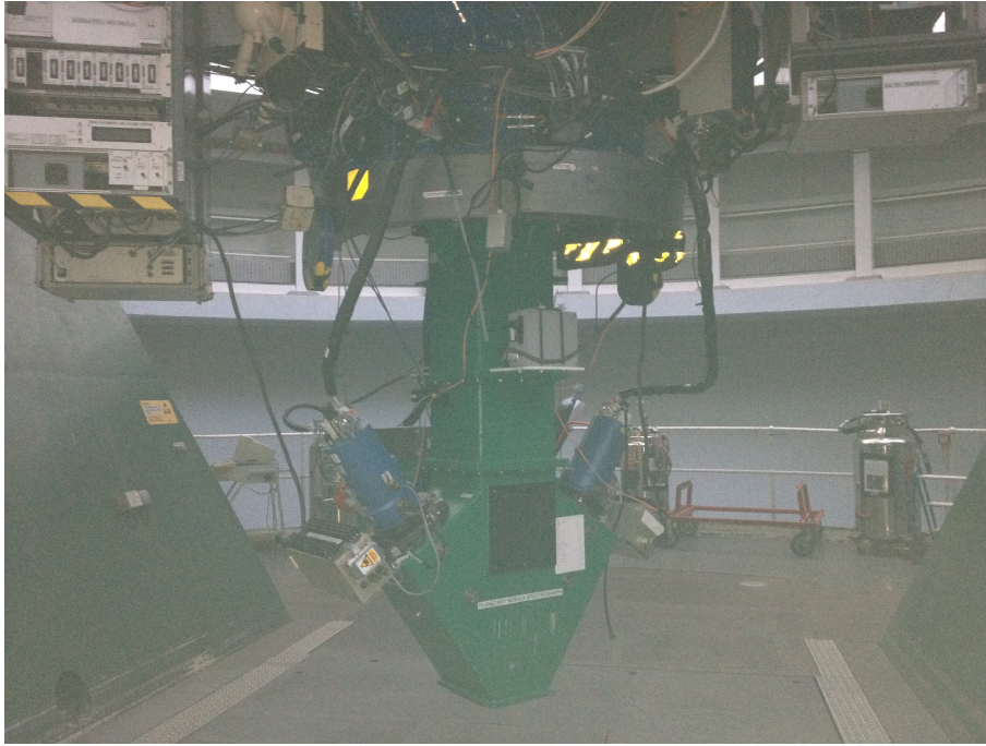
Figure 2.2: Actual PN.S instrument. The light comes from above and is dispersed towards the blue arms on the sides, reaching two CCDs at the end of each one. Credits: Ana Chies Santos.
