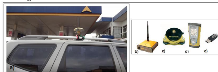
Figure 4: Kia Mohave vehicle (a), GNSS receptor (b) and accessories (d and e) used during the kinematic GNSS survey.
