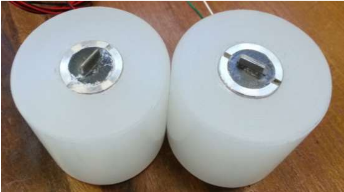
Figure A.24: Bench BE modules positioned in their nylon pedestal
