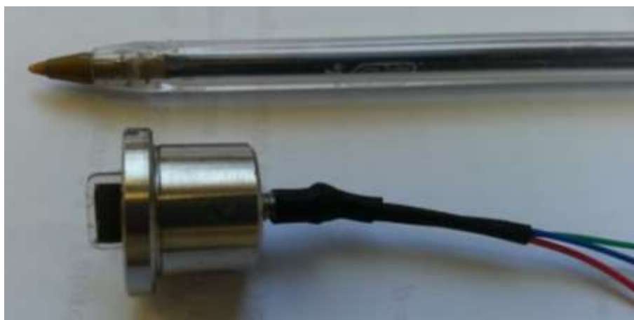
Figure A.23: BE receiver (series connection) with a third wire soldered to the threaded part of the metal case (drain line)
