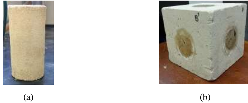
Figure 3.7: Cured Osorio sand/cement specimens – (a) cylindrical specimen (b) cubical specimen.
