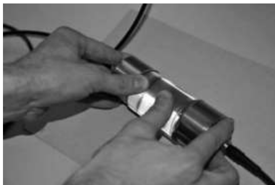
Figure 3.15: Calibration rod positioned for p-waves transducer calibration
