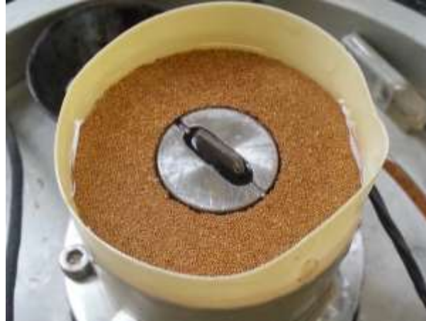
Figure A.37: Porous disk accommodated on the triaxial pedestal
