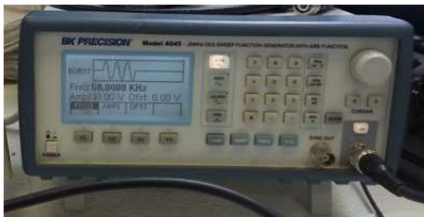
Figure A.7: BK PRECISION® function generator used to create the electrical input signals sent by the BE transmitter
