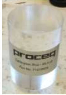
Figure 3.14: Calibration rod of the ultrasound pulse velocity equipment
