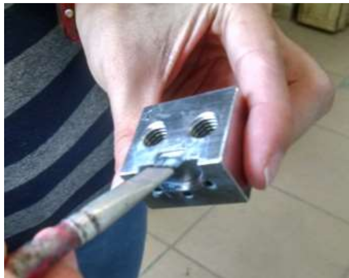
Figure A.19: De-moulding agent (white glue) being applied on the bottom part of the metal mould for BE encapsulating
