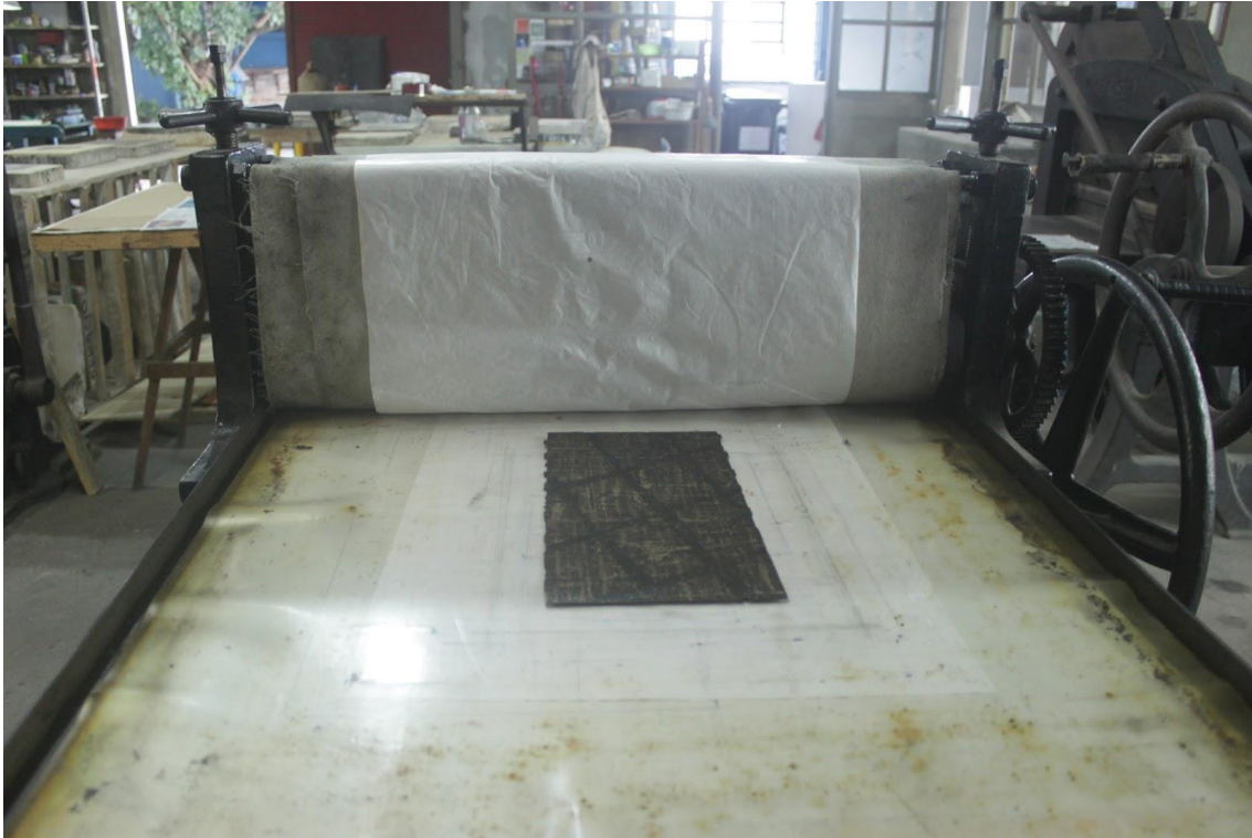
Figure 15: Copper plate in the press. After the dampened paper covers the plate, the first test is ready to be printed.
