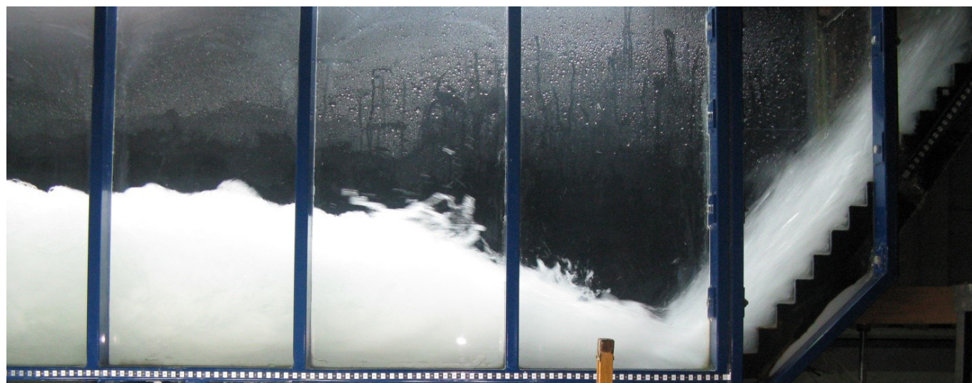
Figure 4. Runoff for the flow of 80 L/s.
