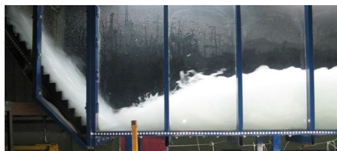
Figure 9. Flow for a discharge of 80 l/s.
