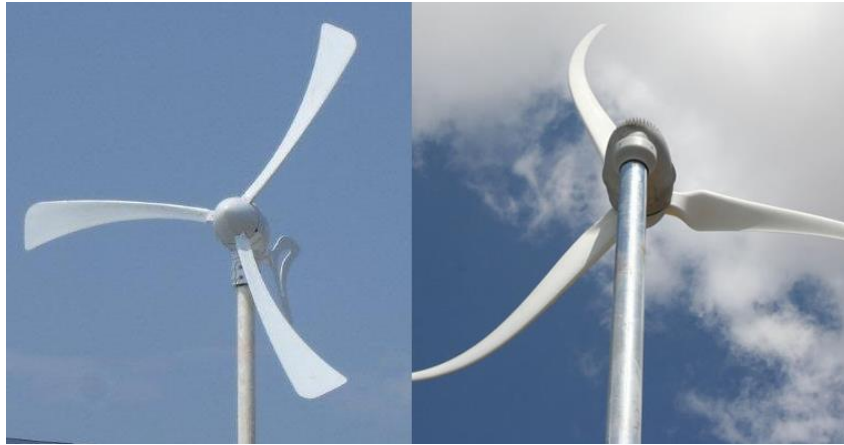
Figure 2.1 – Examples of small turbines with curved blades.
