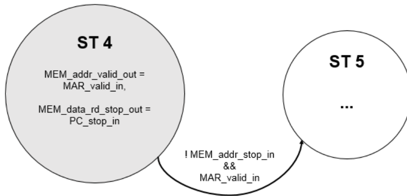
Figure 30 – FSM outputs and transitions from ST5 - STA, LDA, ADD, OR, AND
