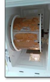
Microwave drying with rotary drum (speed = 60 rpm)
