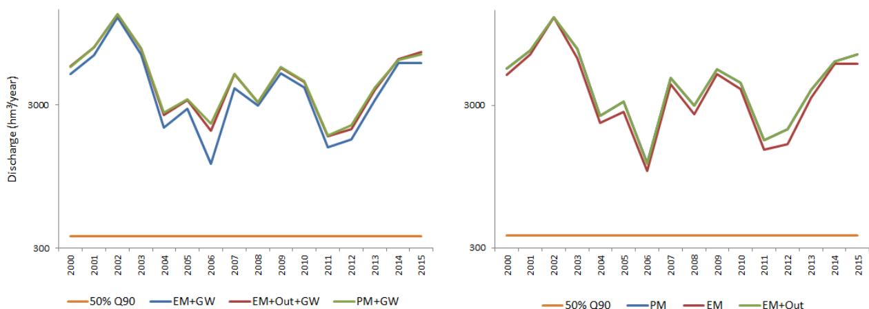
Figure 11. Comparison between the outflows on all simulated scenarios with the limited outflow (50% of the Q90).
