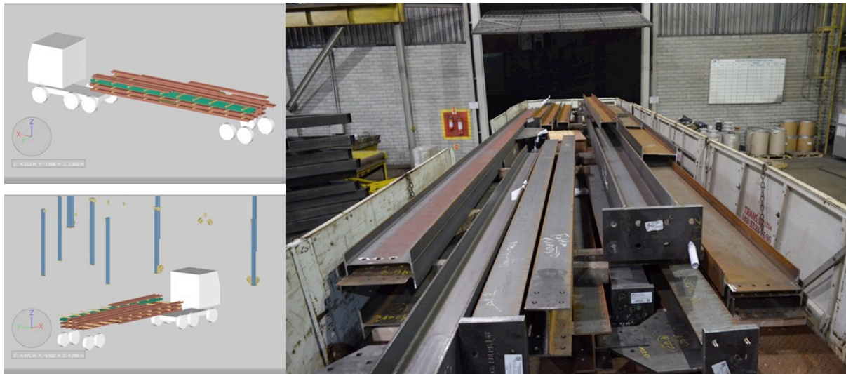
Figure 43: 3D load plan model (left) and actual random load (right)
