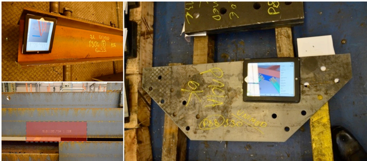
Figure 40: Tracking and matching of sub-components with mobile visualization
