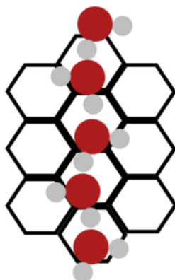
Figure 1.2: Inside the inner of a small carbon nanotube (diameter < 1 nm), water forms the so-called “single-file” structures.
