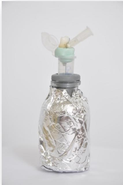
*Figure 1.* Apparatus used for debris extrusion collection.
