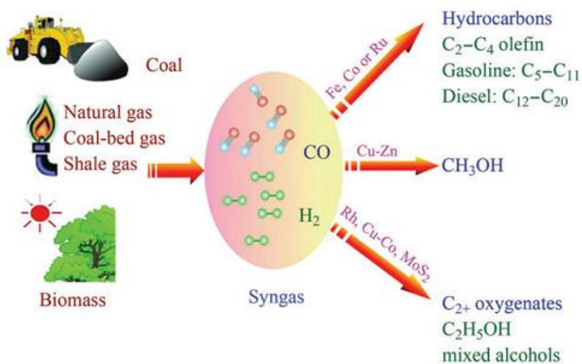
Figure 1.1 Transformation of non-petroleum carbon resources into liquid fuels and chemicals via syngas. Reproduced from Zhang et al. [3].
