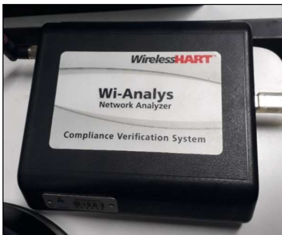
Figura 5: Wi-Analys Network Analyzer, o sniffer do WirelessHART.
