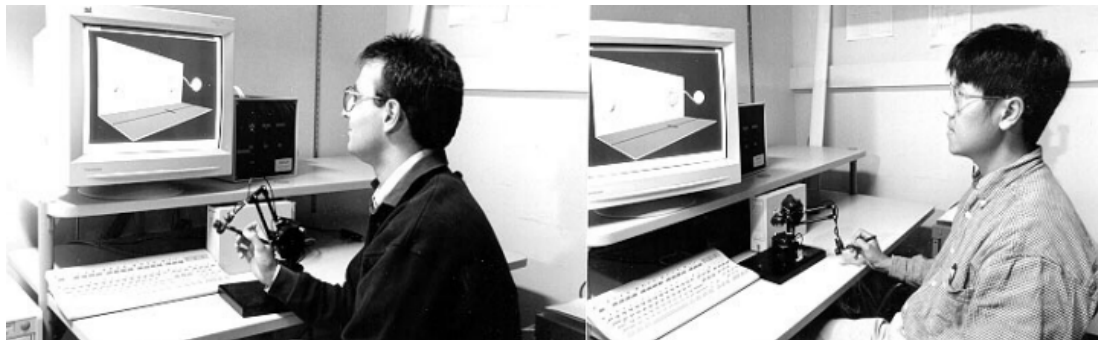
Figure 2.9 - A VR setup that enables two people, at remote locations, to interact with each other through visual and haptic displays
