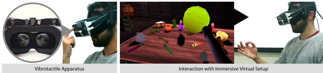
Figure 6.17 - Final experimental setup. (left) Vibrotactile headband and articulatory screen added to the VR headset. (right) Subjects could use their hand to manipulate objects and send vibrotactile cues with gestures in the articulatory screen
