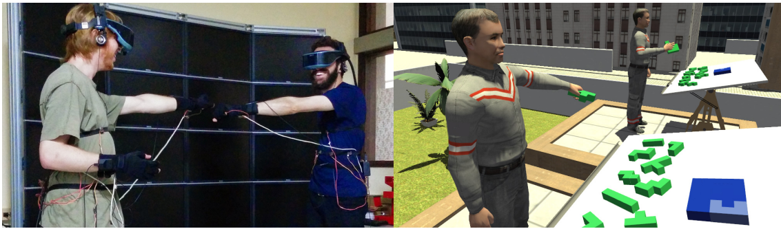
Figure 5.6 - (right) Users wearing the tactile display, data gloves, and the HMD to perform the puzzle assembly. (left) Shared virtual environment
