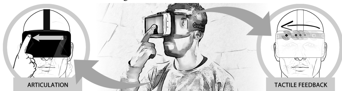
Figure 6.13 - Gestures are captured by the touch surface while the resulting tactile feedback is felt into the HMD through vibrotactile actuators
