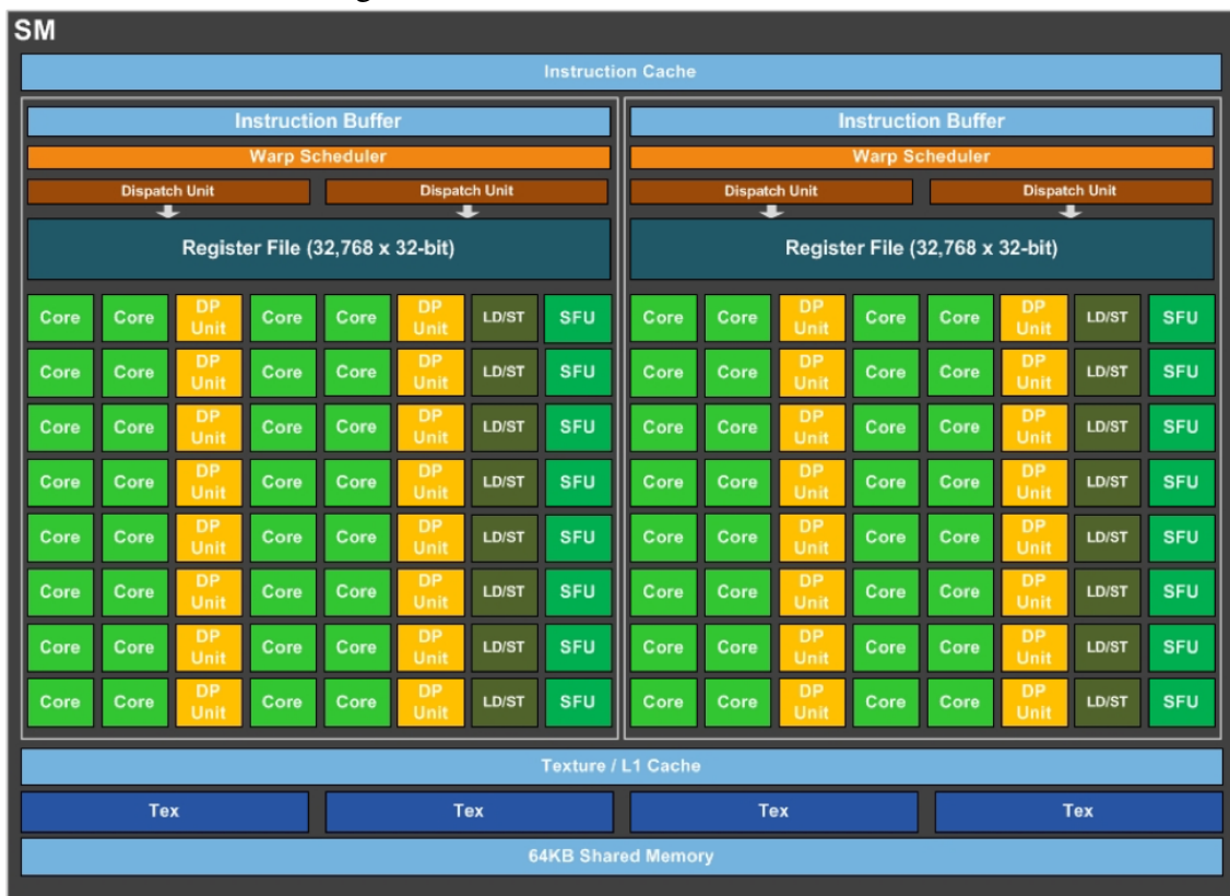
Figure 5.8: Architecture of the Pascal SM.
