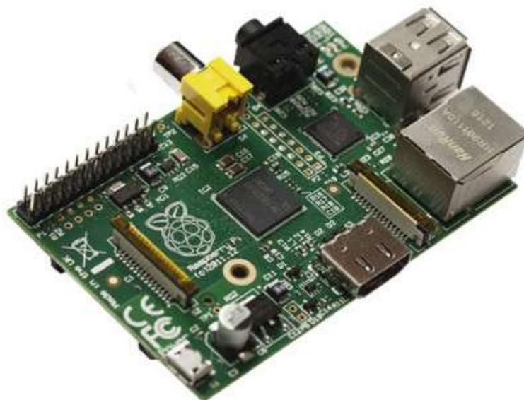
Figura 13 - Raspberry Pi 2, com processador ARM1176JZF-S.
