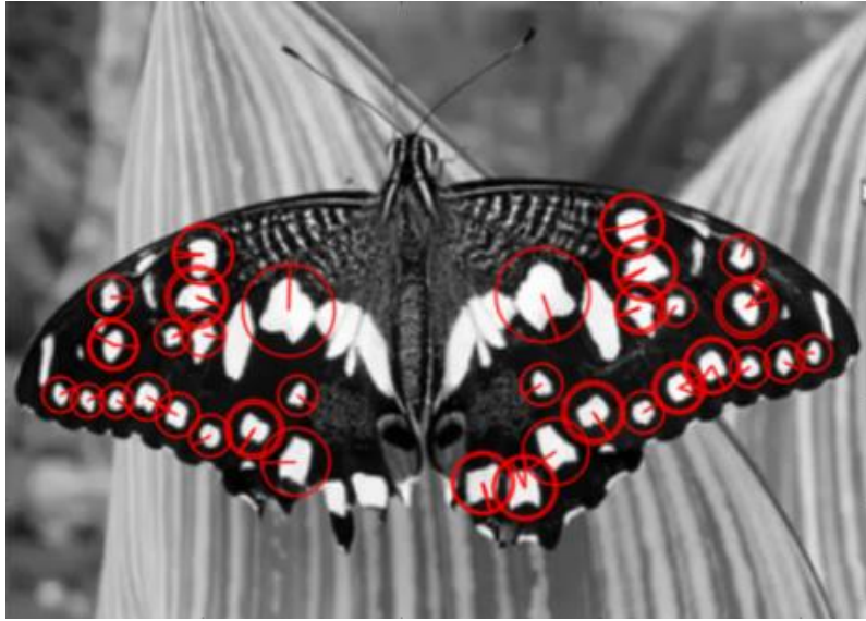
Figure 3.4: Graphical representation of the keypoints selected from an image by the SURF algorithm, shown inside the red circles.
