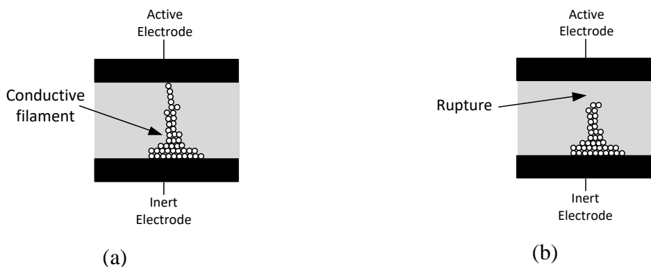
Figure 3.2 – Electrochemical memristive device: (a) RSD in LRS with a CF, and (b) RSD in HRS with ruptured CF.
