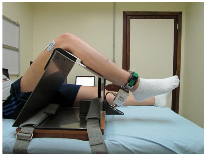
Figure 3.4. Attachment of the stainless steel structure to the stretcher and of the load cell to the distal end of the subject's lower limb.
