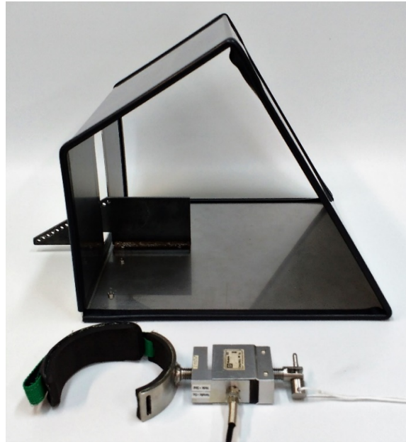
Figure 3.2. Dynamometry system instrumented with a load cell for the evaluation of muscle strength at the intensive care units' beds.
